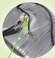
Typical Sender Unit on a fuel tank
